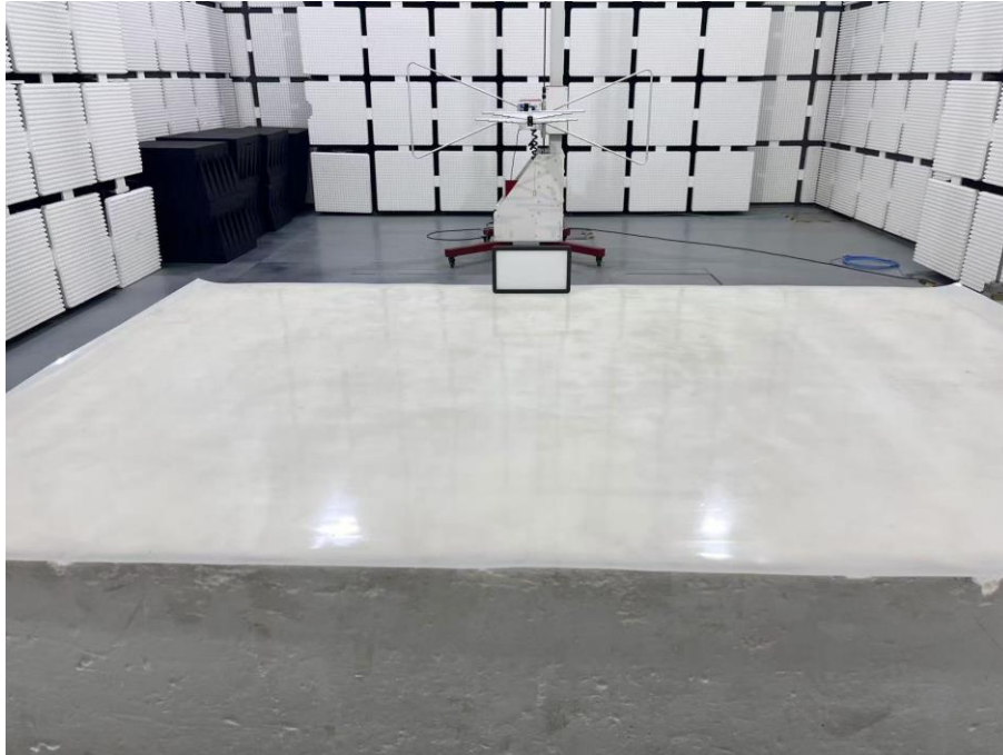
Set-up for Radiated Spurious Emission, Above 1GHz
