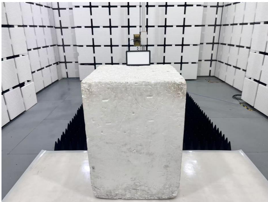
Set-up for Radiated Spurious Emission, Above 1GHz
