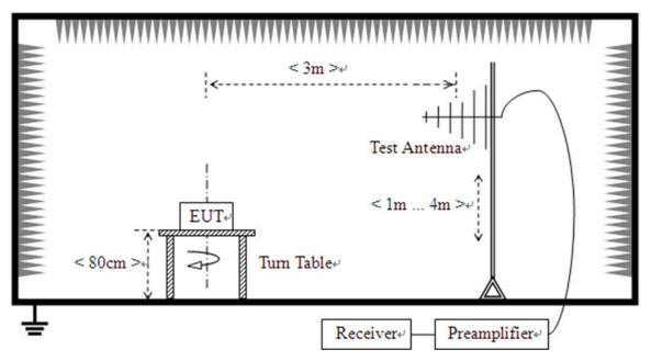
(For the test frequency from 30MHz to1GHz)
