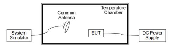
The EUT, which is powered by the DC Power Supply directly, is located in the Temperature Chamber. The EUT is commanded by the System Simulator (SS) to operate at the maximum output power i.e. Power Control Level (PCL) = 5 and Power Class = 4. A call is established between the EUT and the SS via a Common Antenna.
