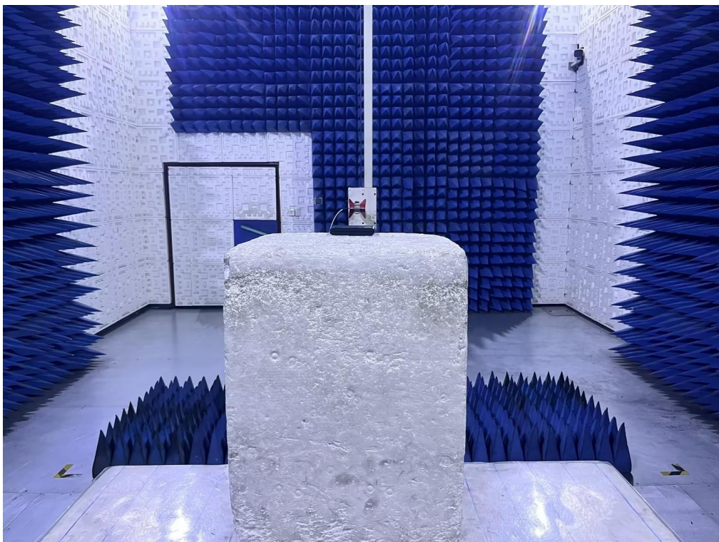
RADIATED EMISSION TEST SETUP ABOVE 1GHz
