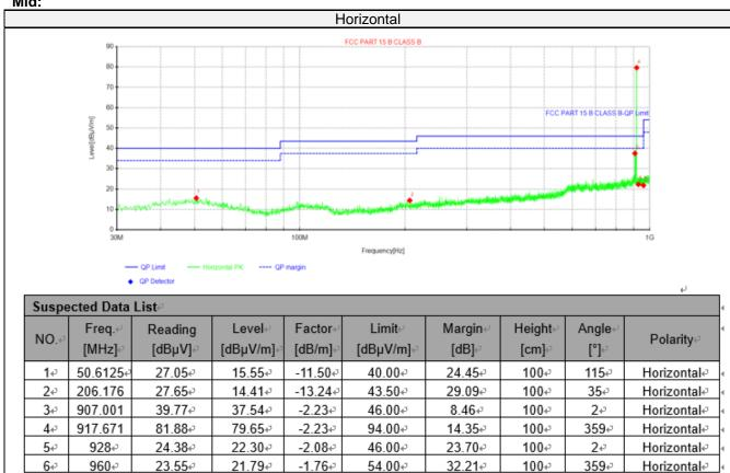
Note:1).Level  $(dB\mu V/m)$ = Reading  $(dB\mu V)$ + Factor (dB/m)
