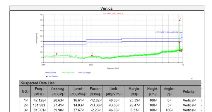
Note:1).Level  $(dB\mu V/m)$ = Reading  $(dB\mu V)$ + Factor (dB/m)
