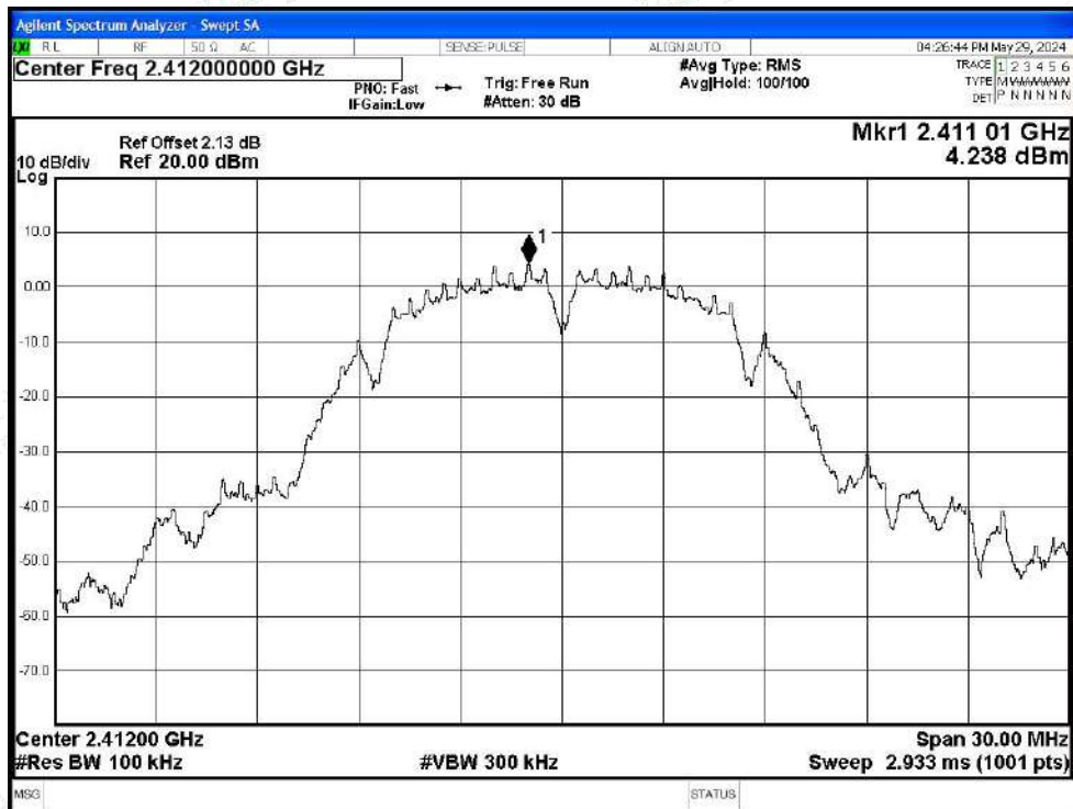
Tx. Spurious NVNT b 2412MHz Ant2 Emission
