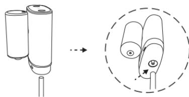
3. Put the sinking bead to Soft pipe.
