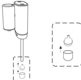
4. Install the Filter foam to Filter Tray, and fit it to water tray up there. (Press and pull it down to remove the foam filter box)
