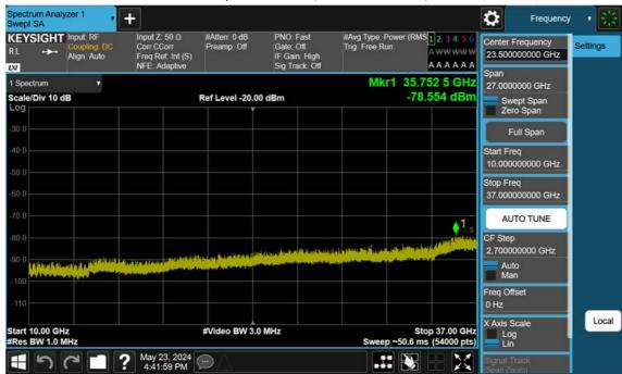
BAND 48. Conducted Spurious Plot 2 (5 MHz Ch. 55265 QPSK RB 1, Offset 0)
