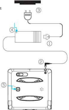
**Important Note:** Please ensure that the machine is continuously powered by AC power while working. The built-in backup battery is prepared to ensure that the machine will not fall off due to sudden power outage during operation, and the duration of the built-in battery is about 20 minutes. If the built-in battery is low, please fully charge the battery before working.
