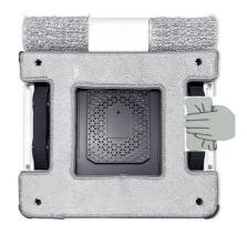
It is recommended that users clean and maintain the belt every time they use the window cleaner (before/after work) to prevent stains, dust, etc. from sticking to the surface of the belt, which may cause abnormal machine operation.
