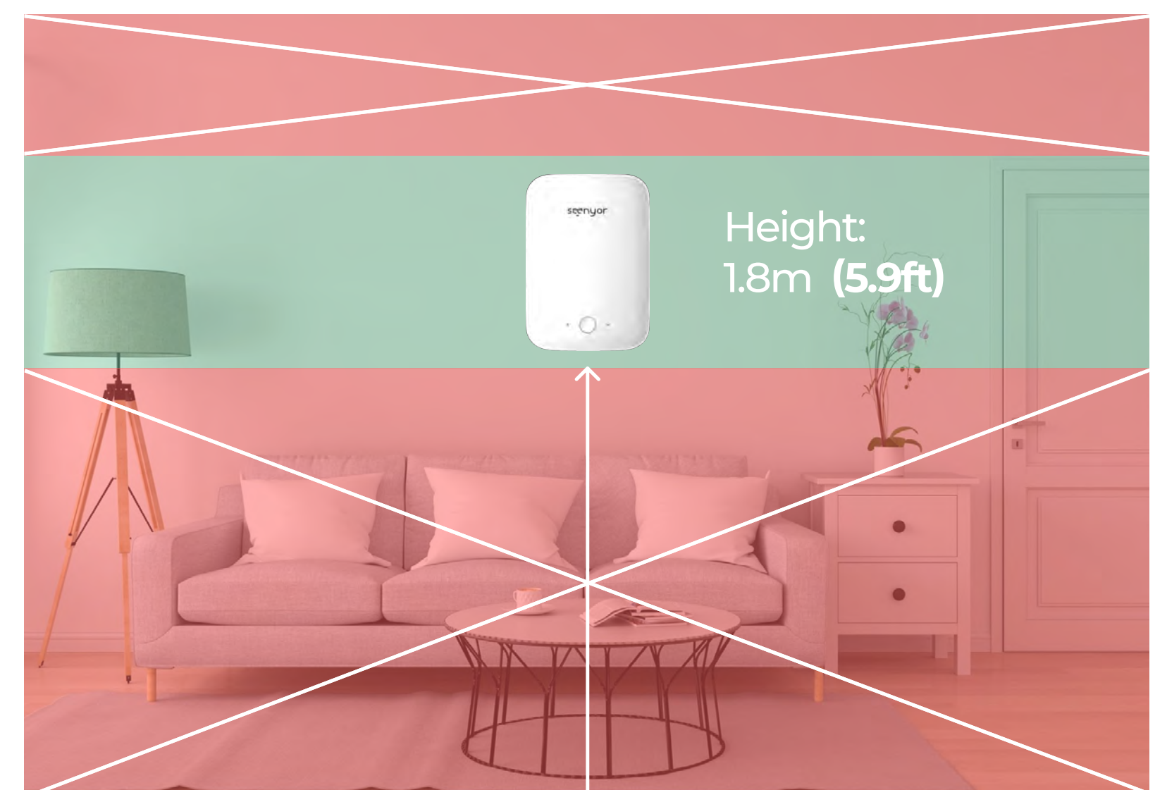
Installation Height MUST BE 1.8m (5.9ft)
