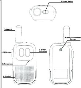
1.Antenna: The antenna for transmitting and receiving signals, don't grab it with your hand when it is working, or it will affect the communication quality.
