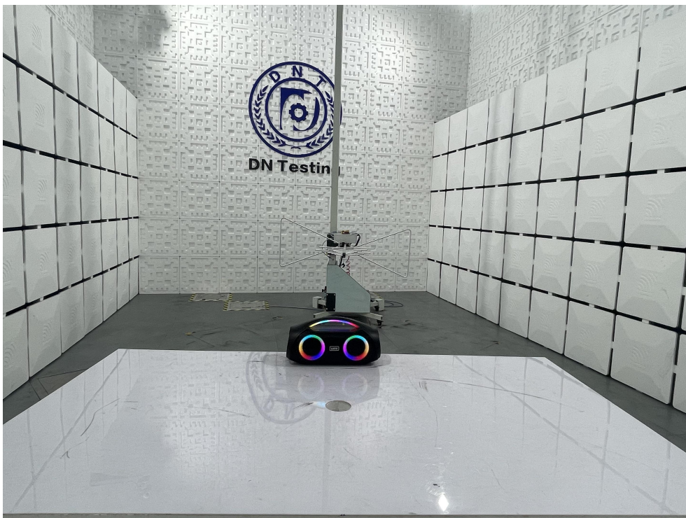
Radiated Emission Test View|(Below 1G)
