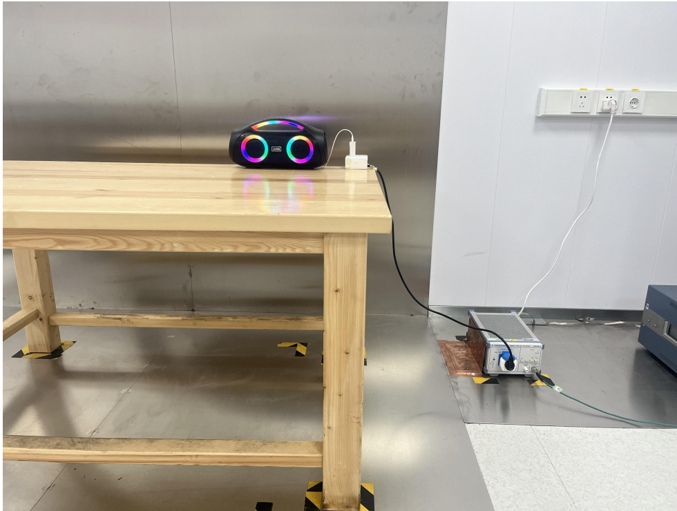
Radiated Emission Test View|(Below 1G)
