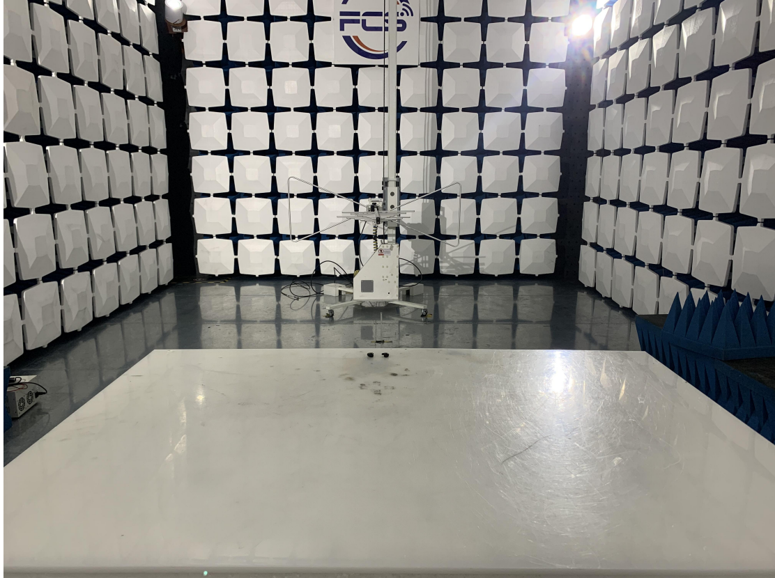
Above 1GHz for radiated emission test setup
