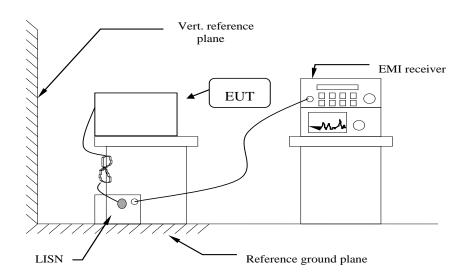
Note: the distance between LISN and Vertical reference plane is 40 cm and the distance between LISN and EUT is 80 cm.
