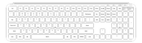
LAYER 3: This layer will be activated when your keyboard's system toggle is switched to Windows and press the fn/MO(3) key.
