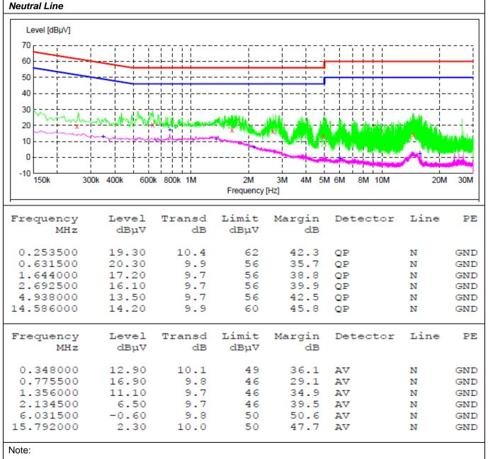
1. Margin(dB)= Limit(dB $\mu$ V) - Level(dB $\mu$ V)
