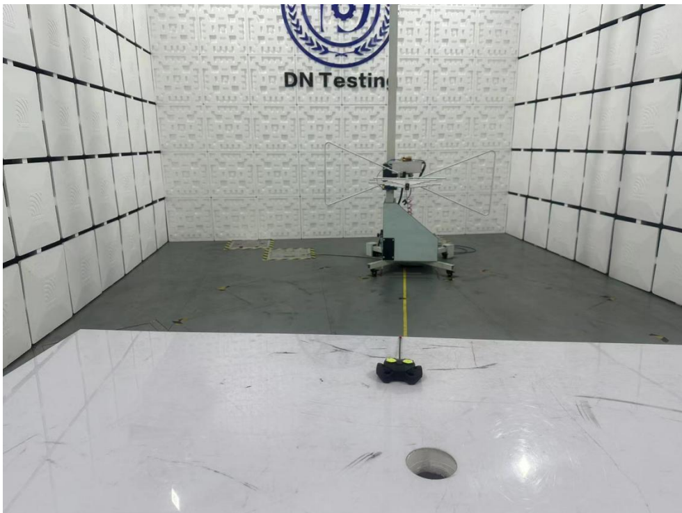
Radiated Emission Test View|(30-1000MHz)
