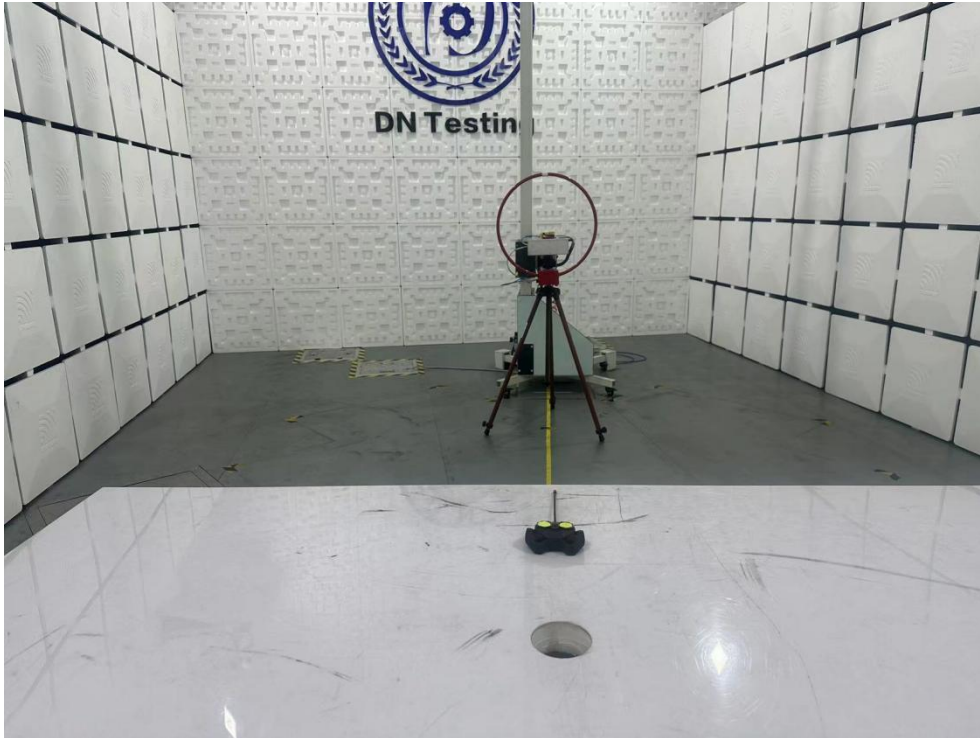
Radiated Emission Test View|(9k-30MHz)
