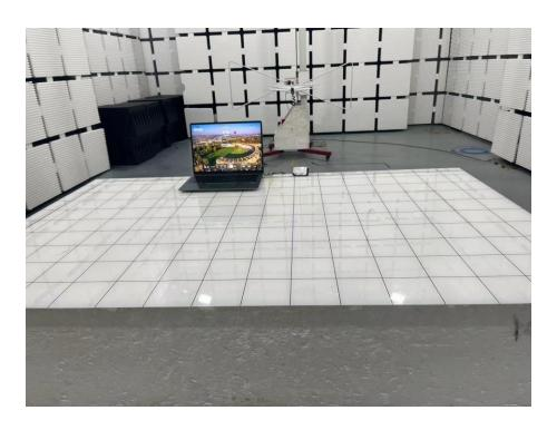
Set-up for Radiated Spurious Emission, Above 1GHz
