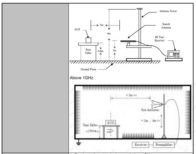
1. For the radiated emission test below 1GHz:
