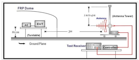
1GHz -40GHz Test Setup:
