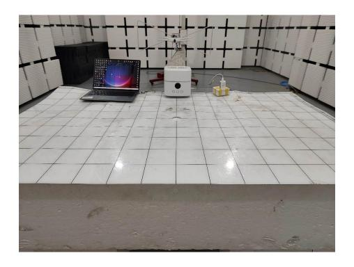
Set-up for Radiated Spurious Emission, Above 1GHz
