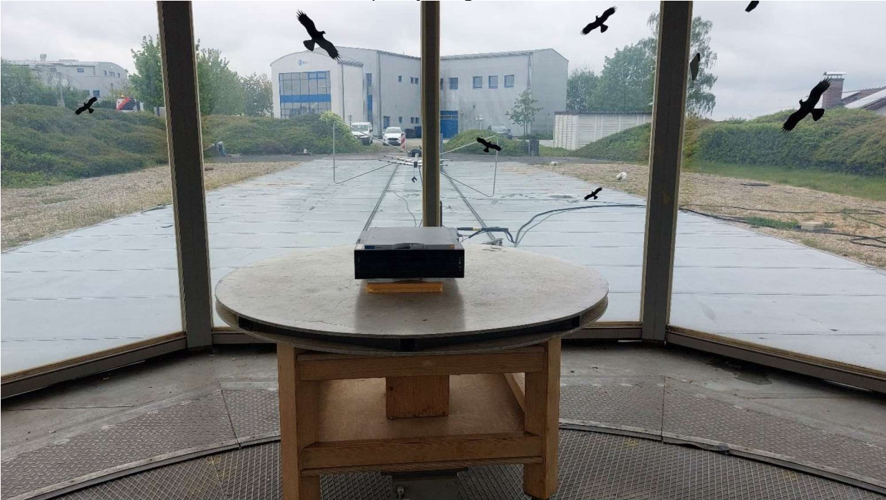
OATS 1 – Frequency Range: 30 MHz to 1 GHz
