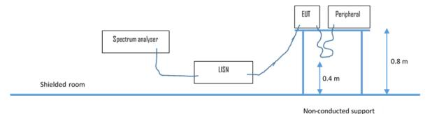
The final level, expressed in  $dB_{\mu}V$ , is arrived at by taking the reading directly from the Spectrum analyser. This level is compared to the limit.
