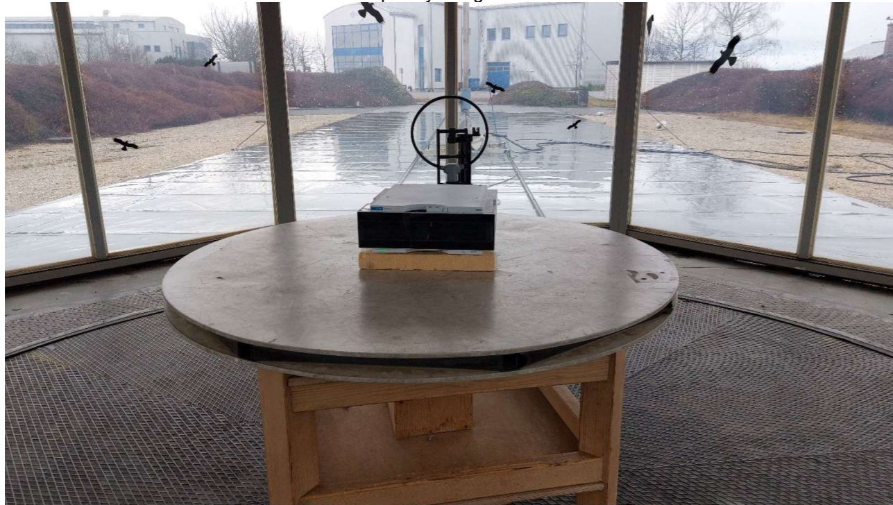
OATS 1 – Frequency Range: 9 kHz to 30 MHz
