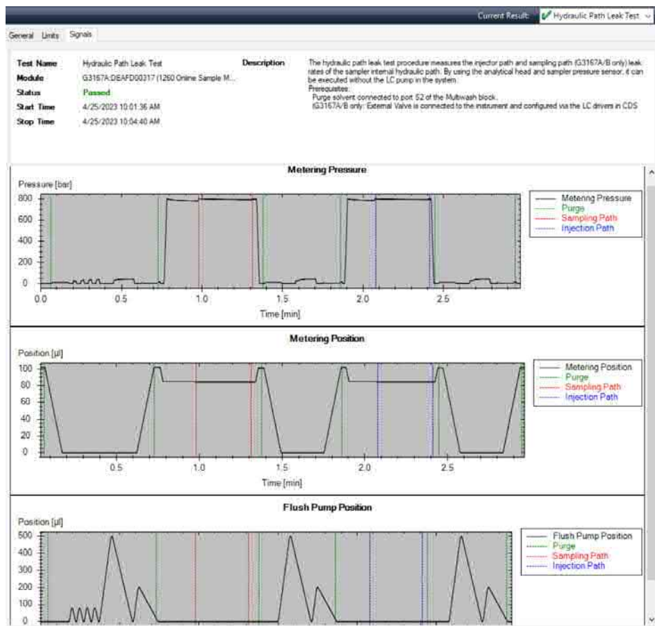
Figure 74 Hydraulic Path Leak Test passed
