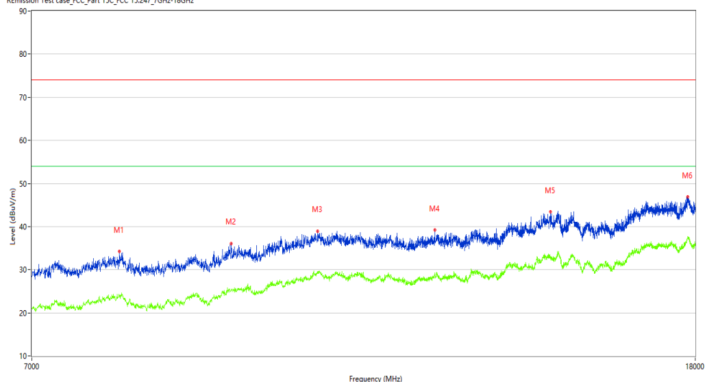
REmission Test case_FCC_Part 15C_FCC 15.247_7GHz-18GHz
