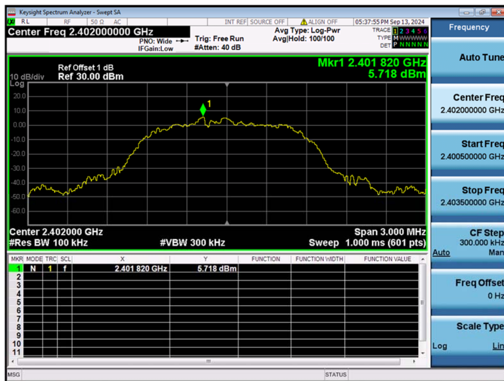
Figure 25: Conducted Spurious Emission & Authorized-band band-edge, 2402MHz, 8-DPSK Carrier Level
