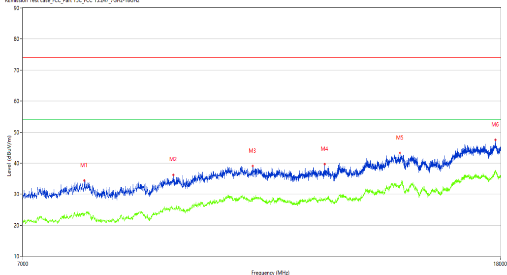
REmission Test case_FCC_Part 15C_FCC 15.247_7GHz-18GHz
