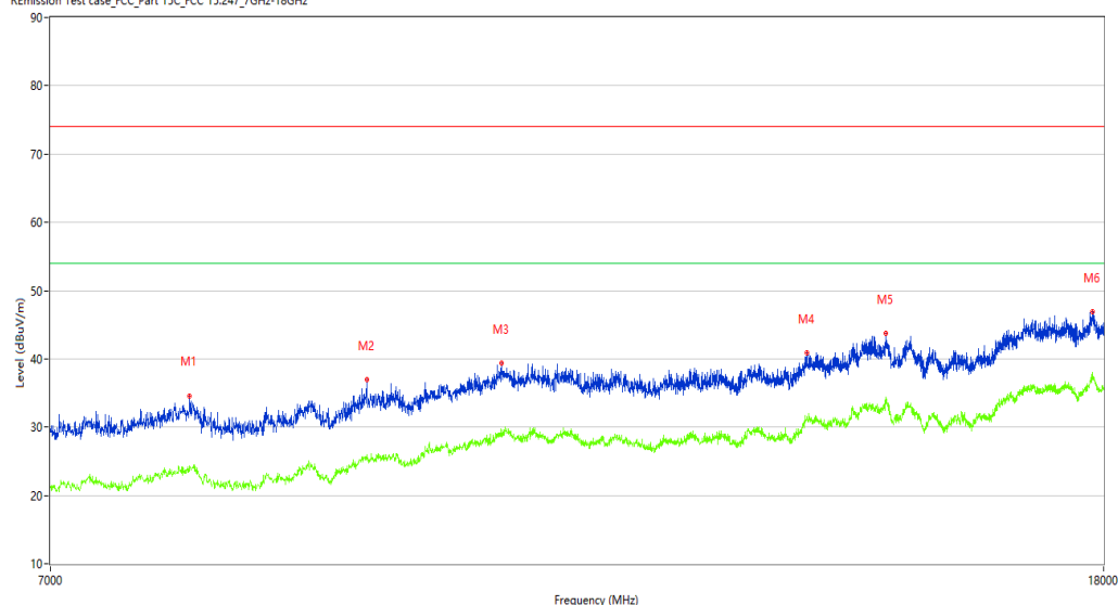
REmission Test case_FCC_Part 15C_FCC 15.247.7GHz-18GHz
