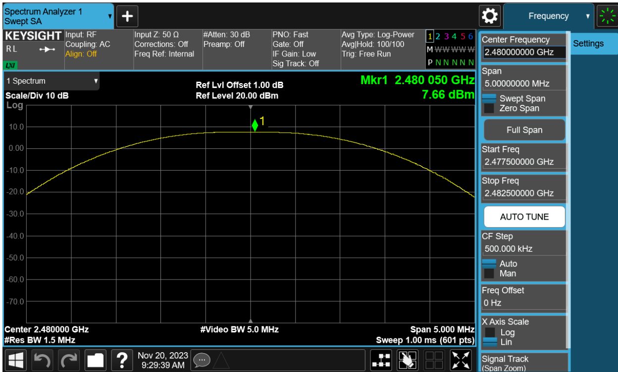
Figure 3: Peak Output Power, 2480MHz
