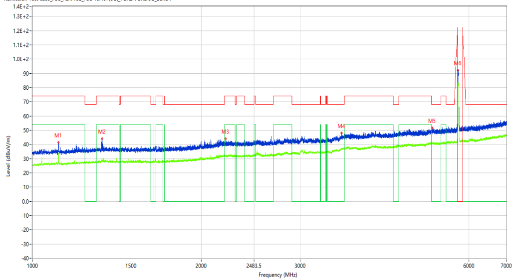
REmission Test case_FCC_Part 15E_FCC 15.407(5G)_1GHz-7GHz 5G_Band4
