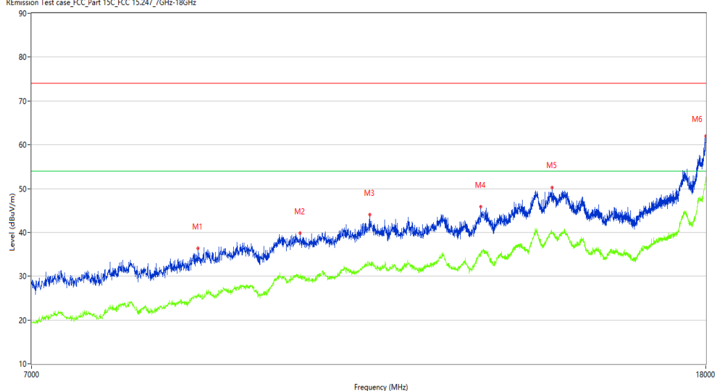
REmission Test case_FCC_Part 15C_FCC 15.247_7GHz-18GHz
