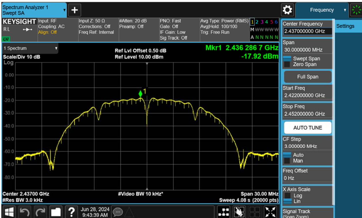
Figure 14: Power Spectral Density, 802.11b, 2437MHz
