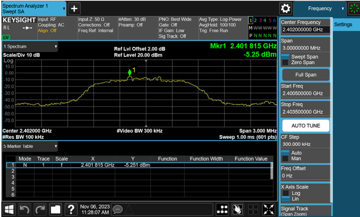
Figure 25: Conducted Spurious Emission & Authorized-band band-edge, 2402MHz, 8-DPSK Carrier Level
