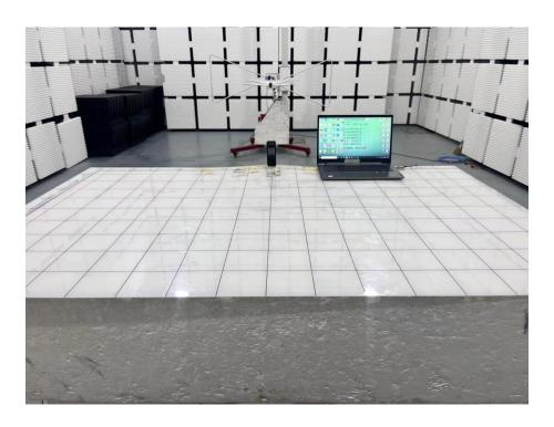
Set-up for Radiated Spurious Emission, Above 1GHz
