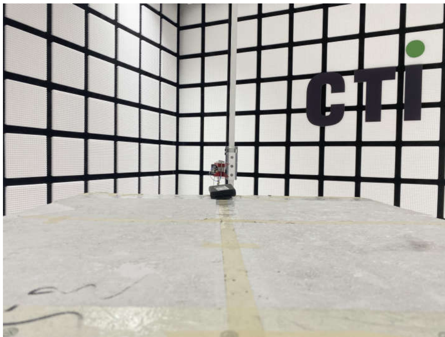
Radiated spurious emission Test Setup-3(Above 1GHz)
