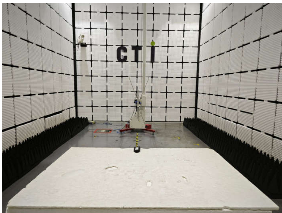
Radiated spurious emission Test Setup-2(Below 1GHz)
