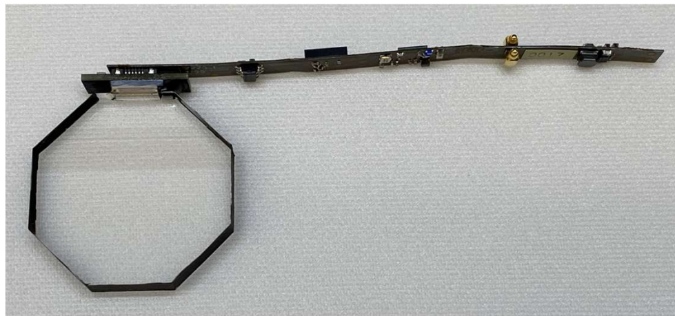
Flex board mated to beamsplitter and display assembly
