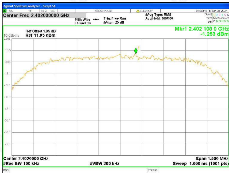
Tx. Spurious NVNT 3-DH5 2402MHz Ant1 Ref
