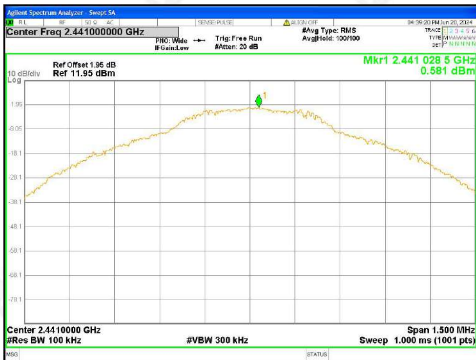
Tx. Spurious NVNT 1-DH5 2441MHz Ant1 Ref
