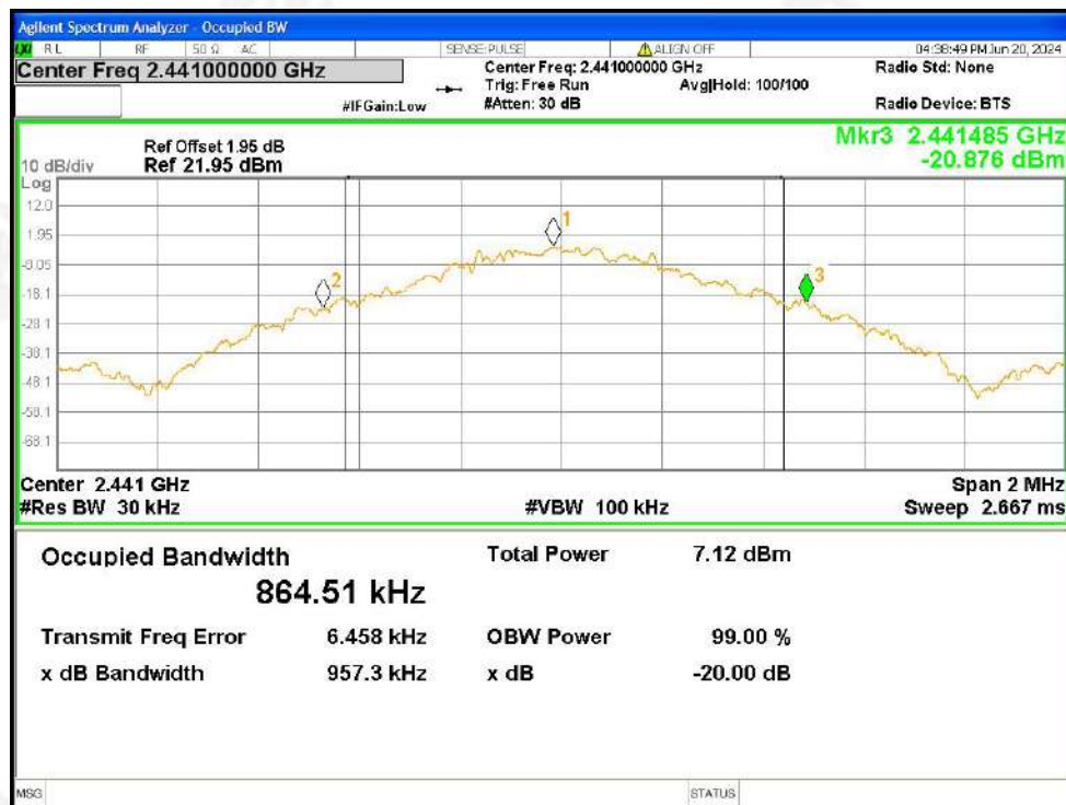
-20dB Bandwidth NVNT 1-DH5 2441MHz Ant1
