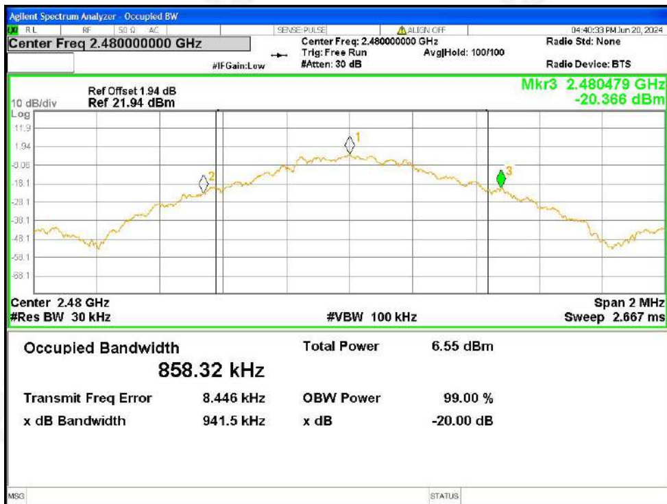
-20dB Bandwidth NVNT 1-DH5 2480MHz Ant1
