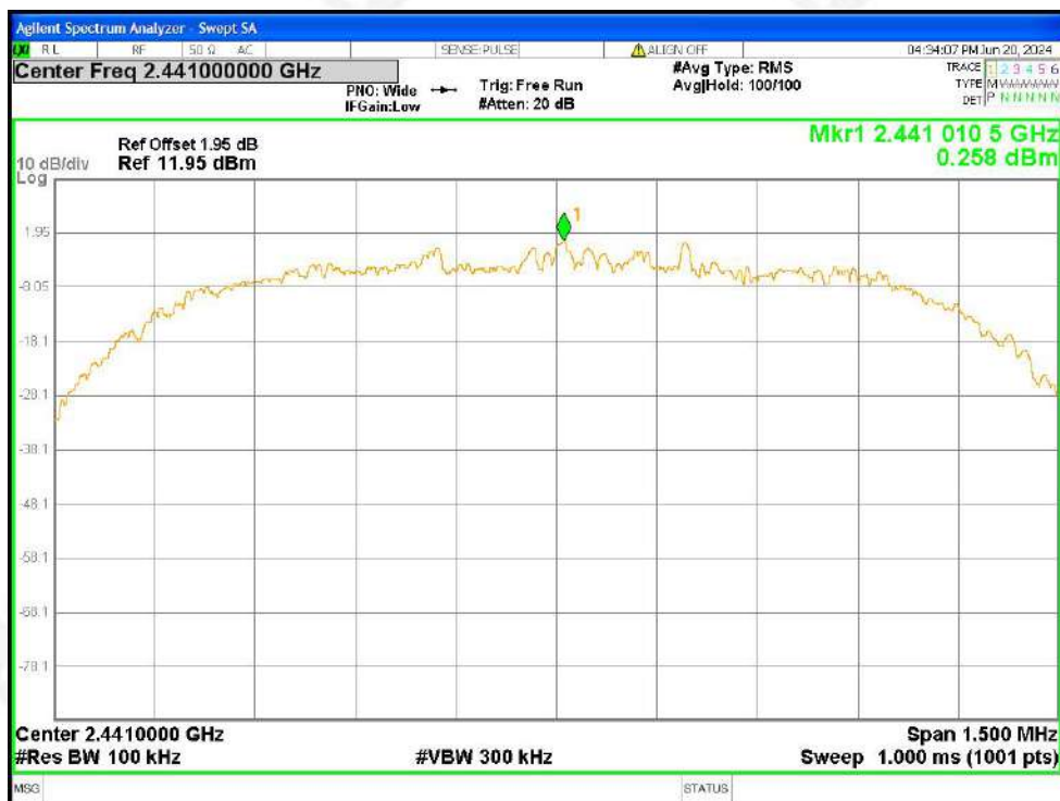
Tx. Spurious NVNT 3-DH5 2441MHz Ant1 Ref
