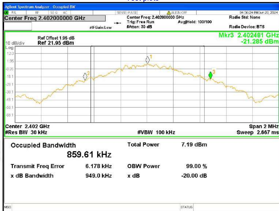
-20dB Bandwidth NVNT 1-DH5 2402MHz Ant1
