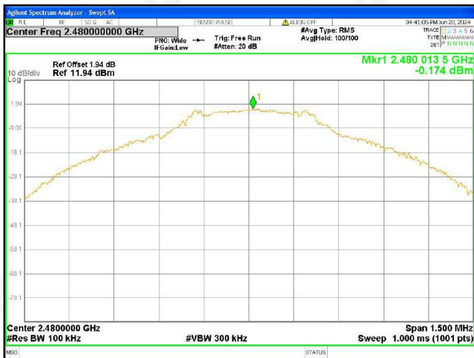
Tx. Spurious NVNT 1-DH5 2480MHz Ant1 Ref
