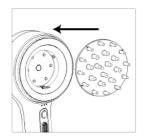
Install the glow secondary blast small coffee box for liquid guiding glow, hold the comb tooth clockwise twist 45° puncture the internal sealing film, long press the power
