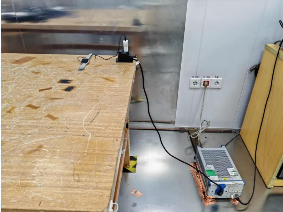
Photo of Setup for Radiated Emission (30MHz~1GHz)
