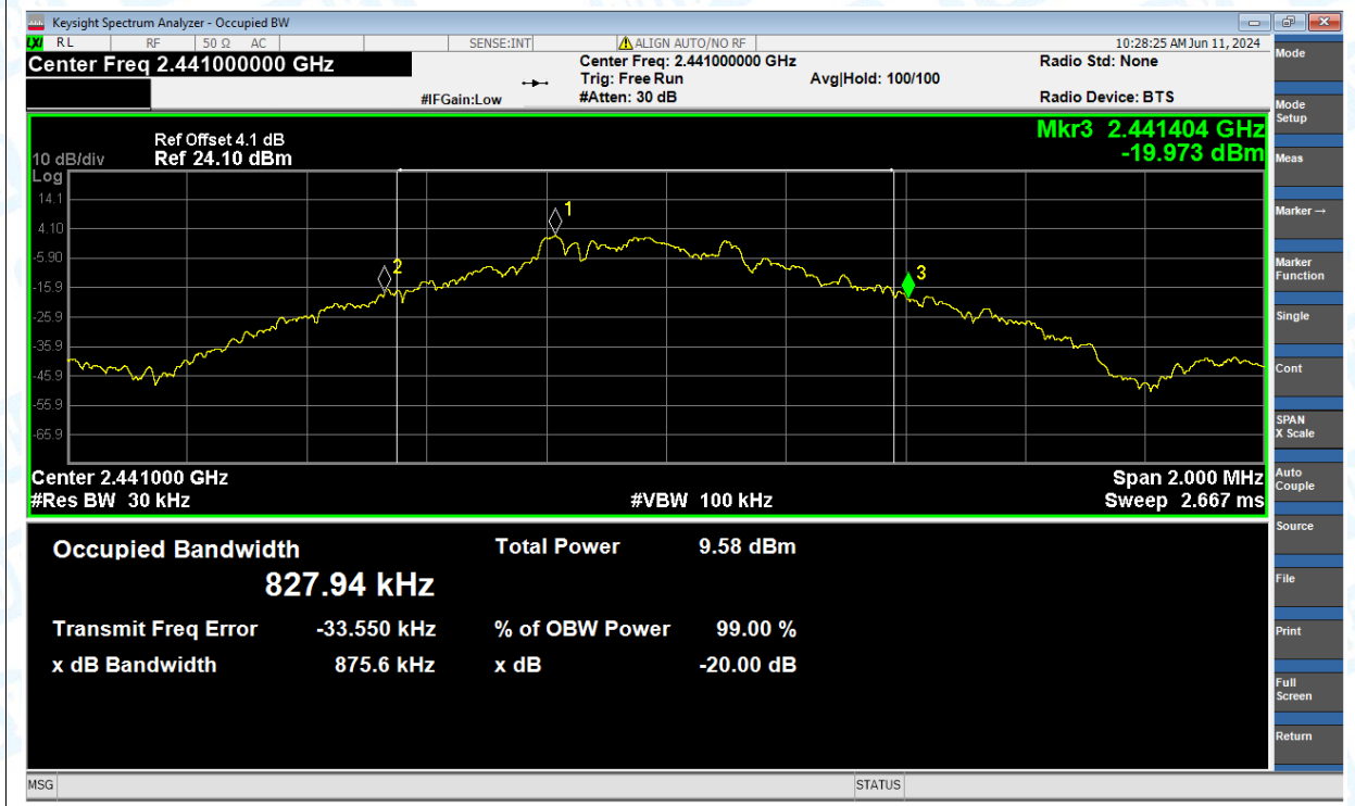
-20dB Bandwidth NVNT 1-DH1 2441MHz Ant1
