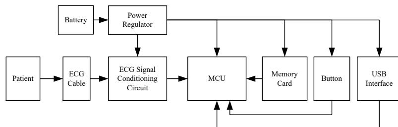
**Electrical Principle Block Diagram of the Recorder**
