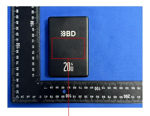
Magnetic Wireless Power Bank Model: KR-W0021 FCCID:2BG4L-KR-W0021 Battery Capacity: 12000mAh Type-C Input/Output: 5V---3A 9V---2.22A 12V---1.67A
