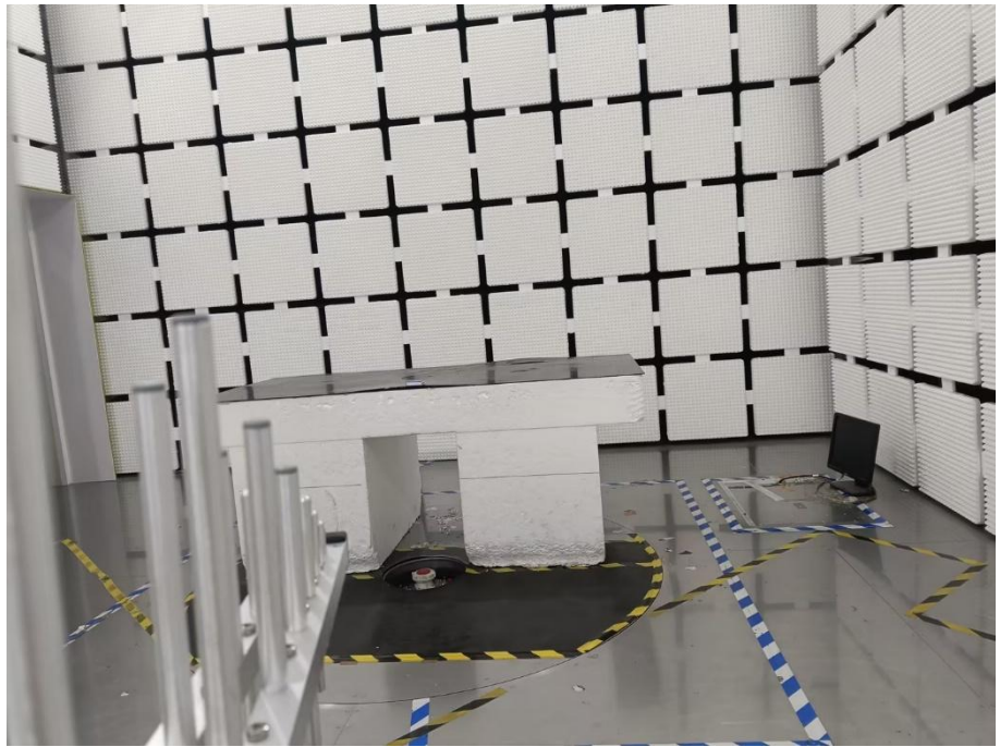
Radiation Emission Test Setup (30MHz to 1GHz)
