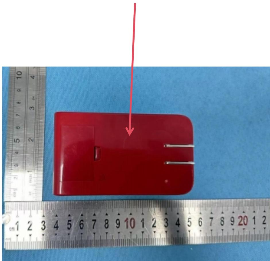
Note: The label is printed on the product by means of Spray paint.
