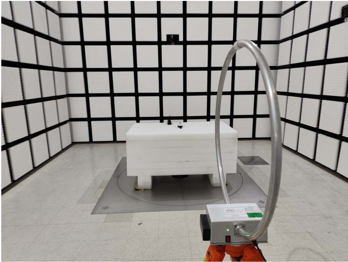
Radiated Emission 9 kHz-30 MHz Perpendicular View
