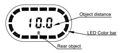
(3) Display will provide audible and visible warnings: The display will show the distance of the detected object, and provide warning beep, according the warning section; the warning sections are equally divided into 5 stages. Take the max. detection as 10m, the warning sections will be divided as below:
