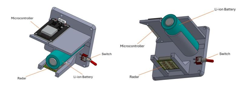
When the switch is flipped up to the "On" position, LEDs on the Microcontroller will light up. The device is programmed so that as soon as it is powered, both the Bluetooth and the Radar will immediately begin radiating energy in their respective wavelengths.
