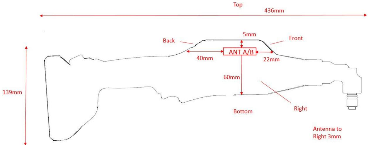
**NX\_-P SAR exclusion calculations for WiFi-SISO and Bluetooth for antenna < 50mm from the user :**
