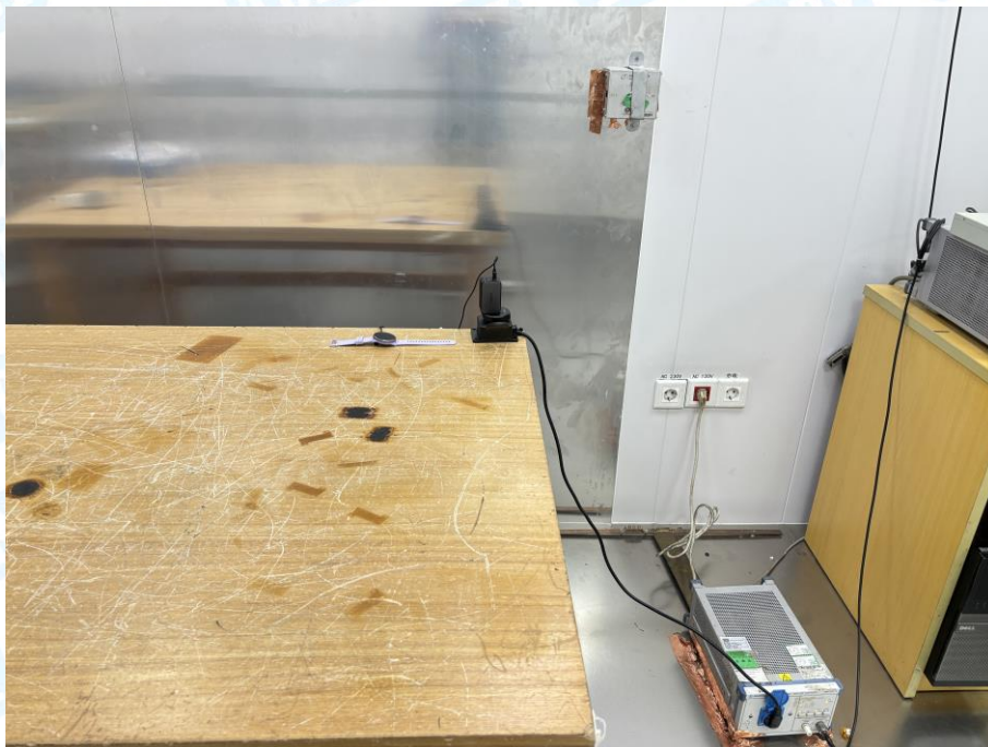
Photo of Setup for Conducted Emission
