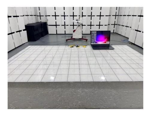
**Set-up for Radiated Spurious Emission, Above 1GHz**
