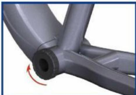
Step 1: Tighten the left headset as shown in the figure. (Tightening torque: 35NM)
