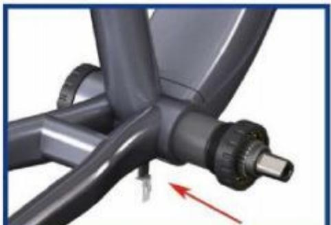
Step 2: Insert the torque sensor assembly through the left side of the bottom bracket, and pull its wire out of the lower hole of the bottom bracket.
