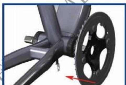
Step 4: Install the crankset until its spline is fitted with that of the torque sensor.
